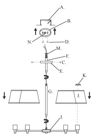
\*\*\*DETERMINE REQUIRED MEASUREMENT BEFORE MAKING CONNECTION-IT MAYBE NECESSARY TO REMOVE SOME OF THE RODS TO OBTAIN THE DESIRED LENGTH\*\*\*
